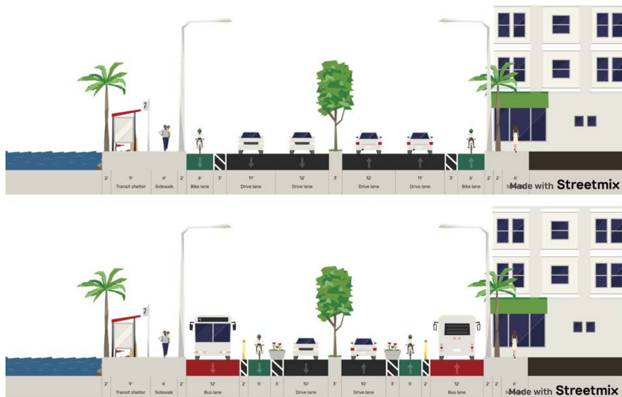
Figure 61: Concept bus-only lane street configuration on El Colegio Rd.
