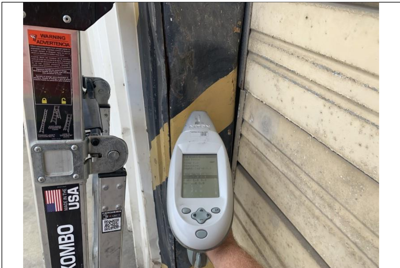
Photo of lead paint on roll-up door frame to Maintenance Shop. Similar yellow stripes are located on the corner support posts of the north canopy structure.
